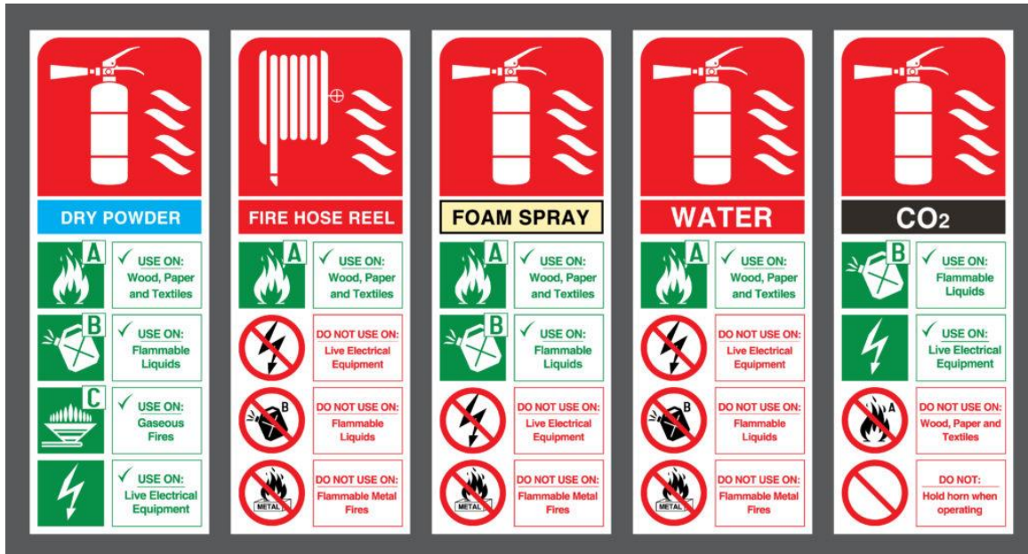
Figure 31: Types of fire extinguishers. Barry. "THE MANY TYPES OF FIRE EXTINGUISHERS." A Total Solution, Inc. Security and Fire Protection, 10 Feb. 2017, www.atotalsolution.com/blog/the-many-types-of-fire-extinguishers/ .
