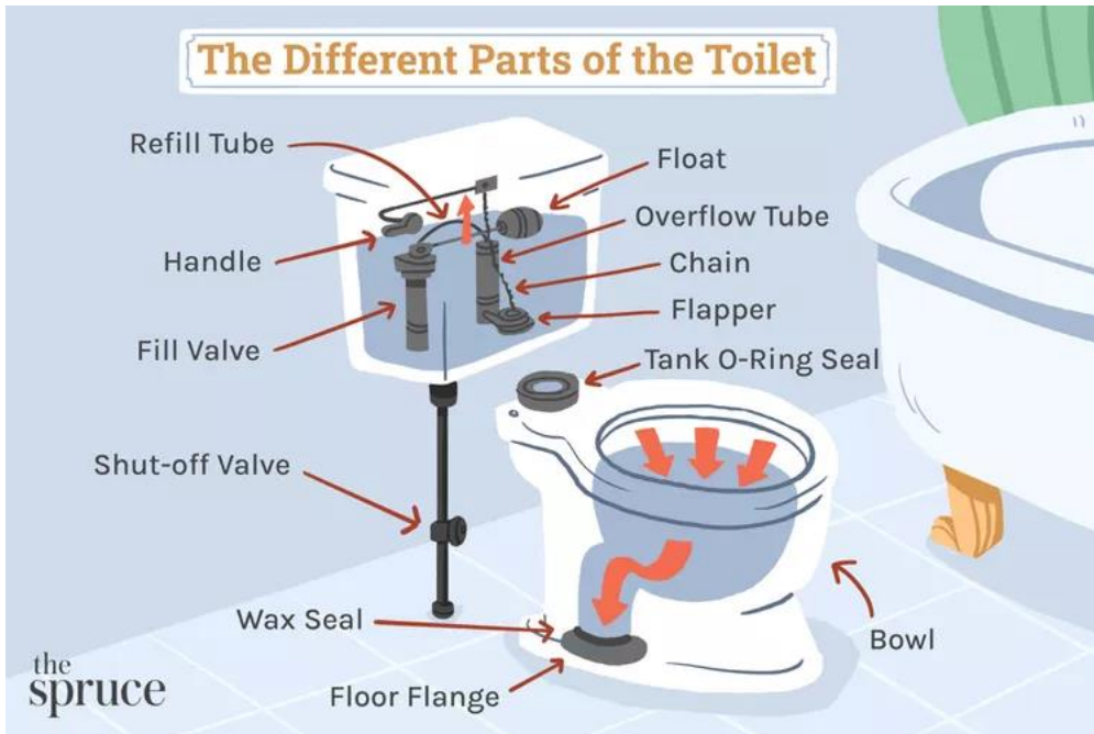
Figure 7: Parts of a toilet. Wallender, Lee. "Parts of a Toilet: What They Are and How to Fix Them." The Spruce, 19 Oct. 2023, www.thespruce.com/the-parts-of-a-toilet-4145300 .
